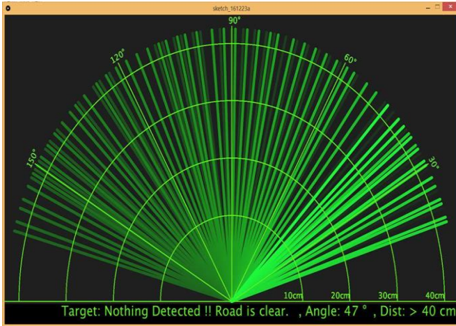
Fig. 8 The output of the ultrasonic in case of clear road
